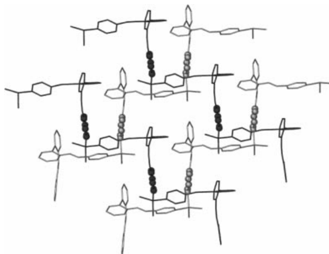
Figure 5. View of \pi-\pi interactions between the adjacent chains along the c axis in 3
